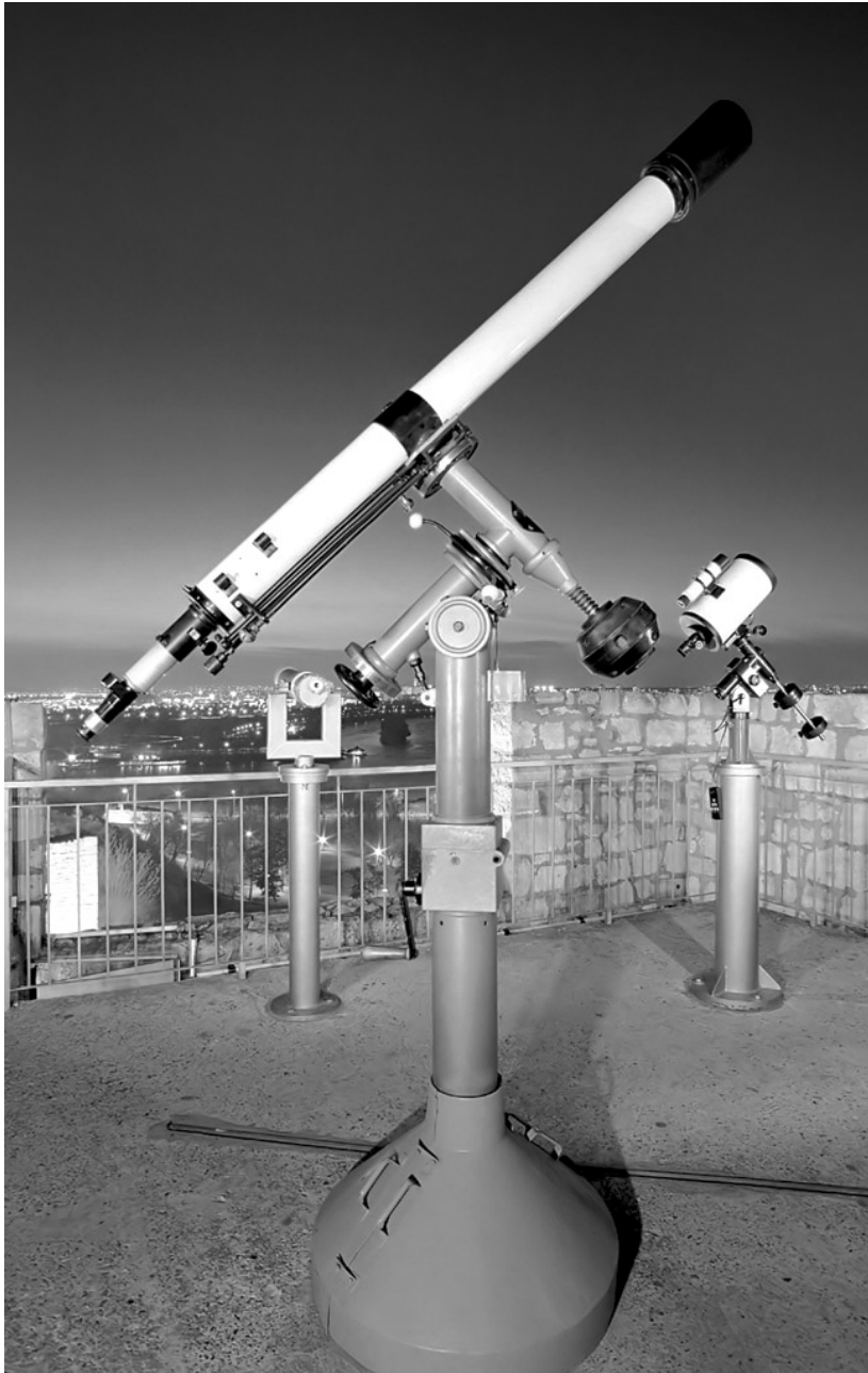
Fig. 5. Two telescopes on the terrace of People's Observatory. In the front is the older one refractor Zeiss (110/2040) and behind the newer one, the reflector TAL-200 K (200/2000). Photo by Vladimir Nenezić.
